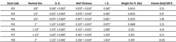
Dimensions are in English units. Tolerances shown are ASTM requirements. CANPEX™ UV PLUS is manufactured to these specifications.
