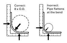
NOTE: Tubing may be bent to a minimum of 5  $\times$  0.D. with approved bend support.
