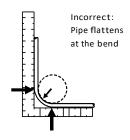
NOTE: Tubing may be bent to a minimum of 5  $\times$  O.D. with approved bend support.
