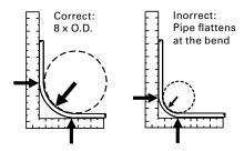
NOTE: Tubing may be bent to a minimum of 5 x O.D. with approved bend support.
