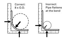
NOTE: Tubing may be bent to a minimum of  $5 \times O.D.$  with approved bend support.
